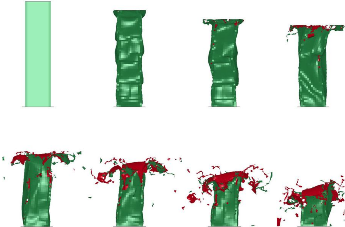
Fig. 20 The Collapse Shape of 15°member in Simulation
