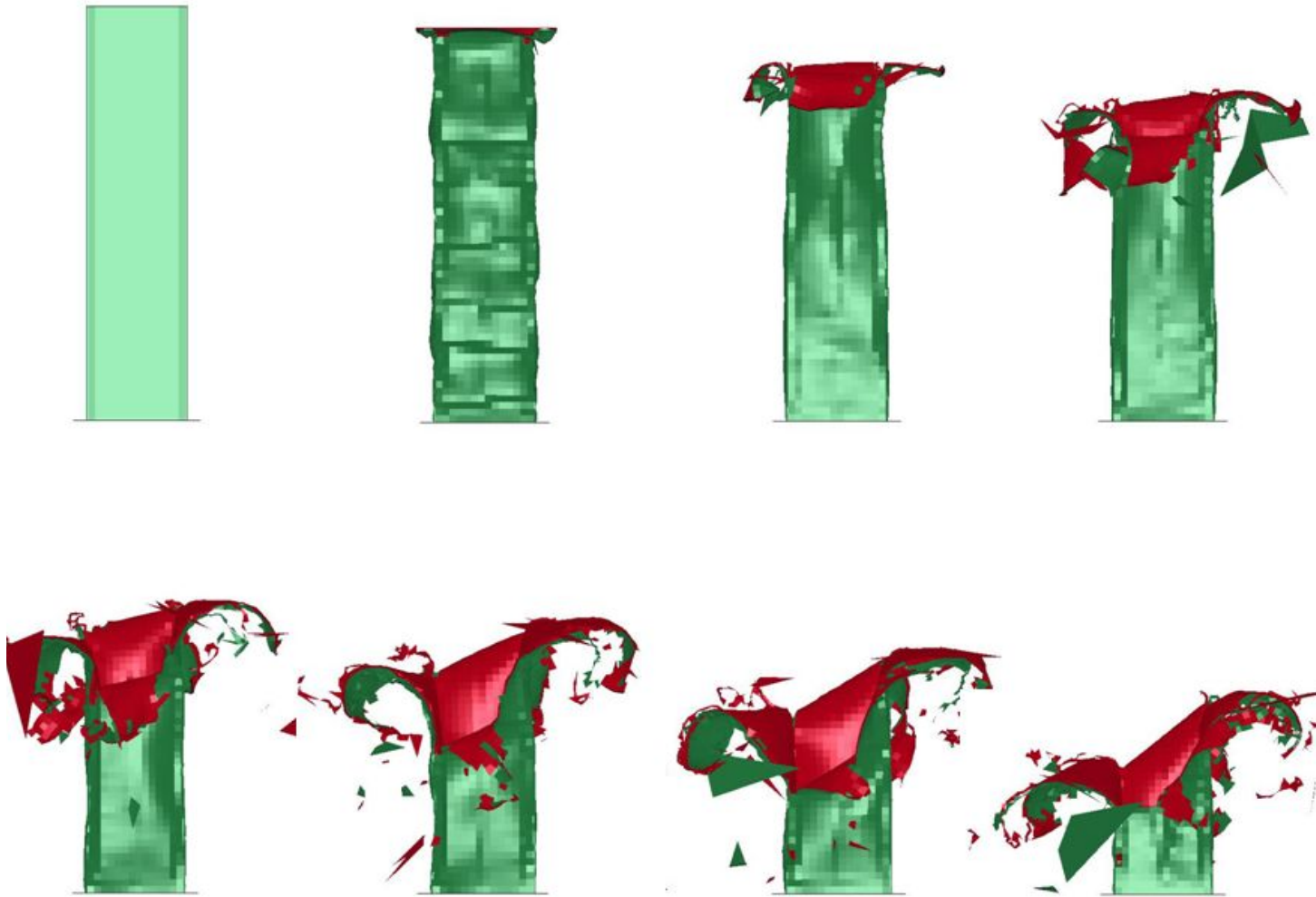
Fig. 22 The Collapse Shape of 45°member in Simulation
