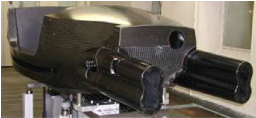
Photo 1 The Volkswagen EcoRacer concept car: (a) complete vehicle, and (b) stripped continuous carbon fiber reinforced composite body structure. 3)
