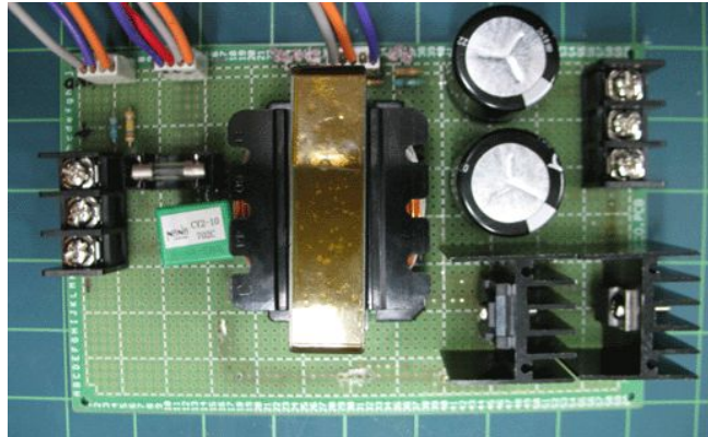
Fig. 5-3 Photo of DC-DC boost converter
