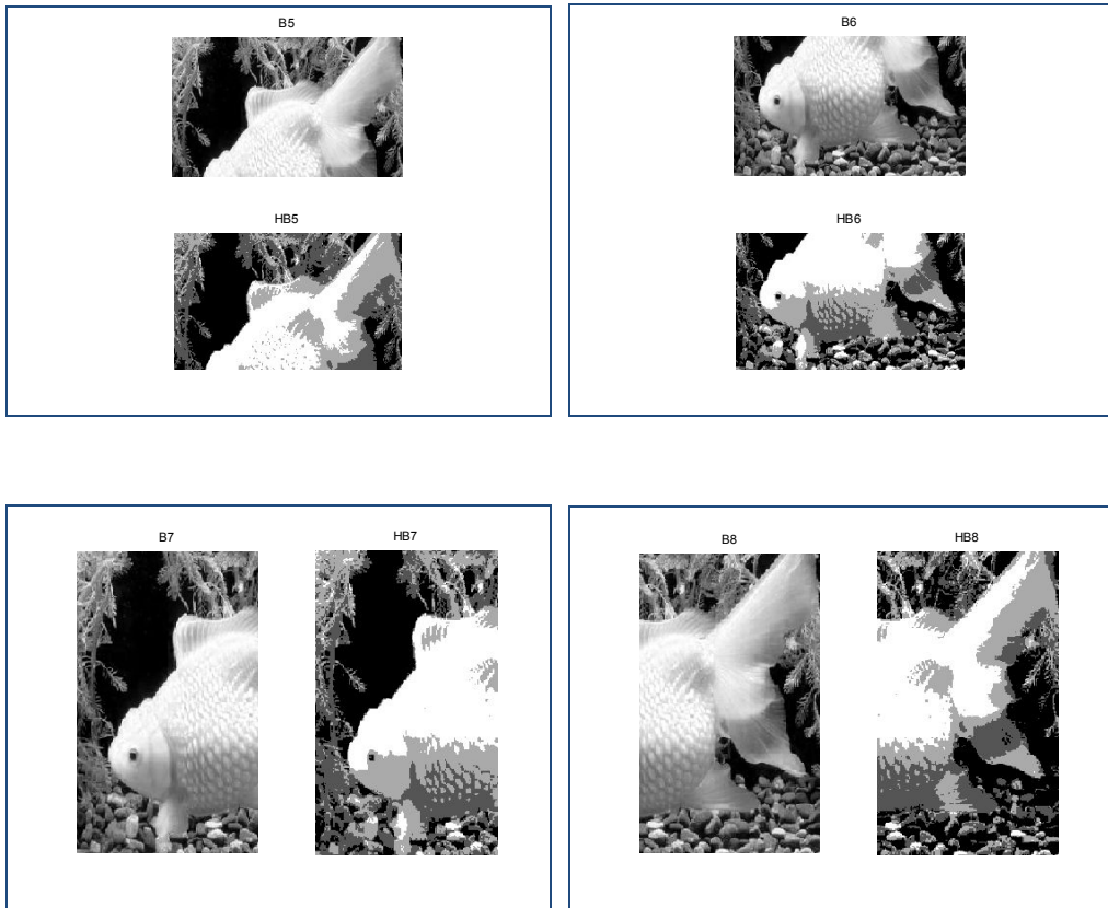
Figure 3.12: (B1~B8) Image blocks (HB1~HB8) Histogram equalized image blocks.
