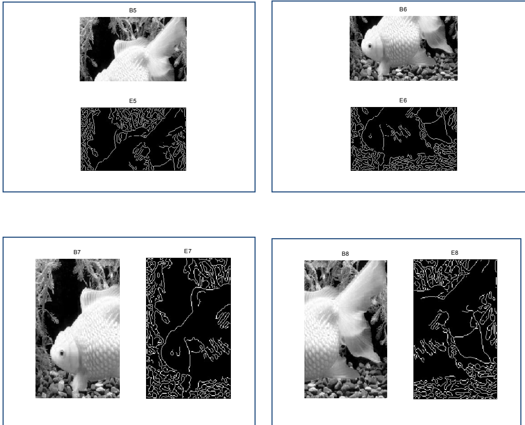
Figure 3.16: Edge detection use 'canny' (B1~B8) Image blocks (E1~E8) Edge image of blocks
