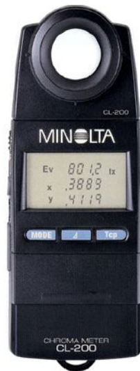
Photo 2.7 Chroma meter(CL-200, Konica minolta sensing Co., Japan)
