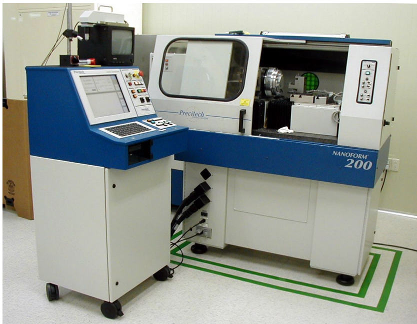
Photo 2.1 Diamond Turning Machine (Nanoform200, Precitech Inc., USA)
