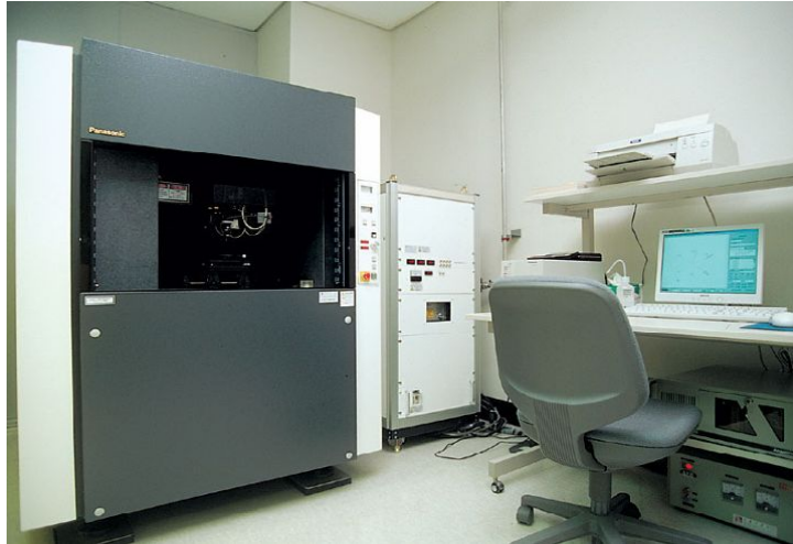
Photo 2.3 Ultra high accurate 3-D profilometer(UA3P, Panasonic Co., Japan)
