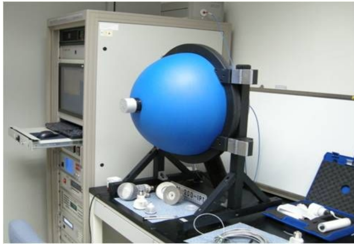
Photo 2.6 Integrating Sphere System(LF Series, PSI Co., Australia)
