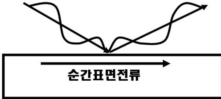
Fig. 5 An apparatus of electromagnetic wave reflection by metal
