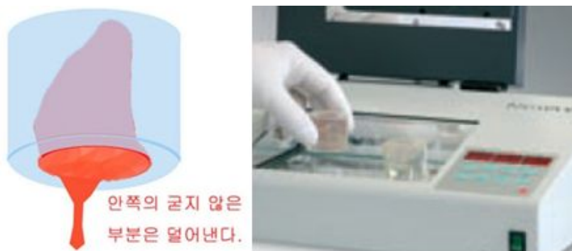
Figure 2 - 7 completely pour the shell material from the investment to make the strong and thin ear shell.
