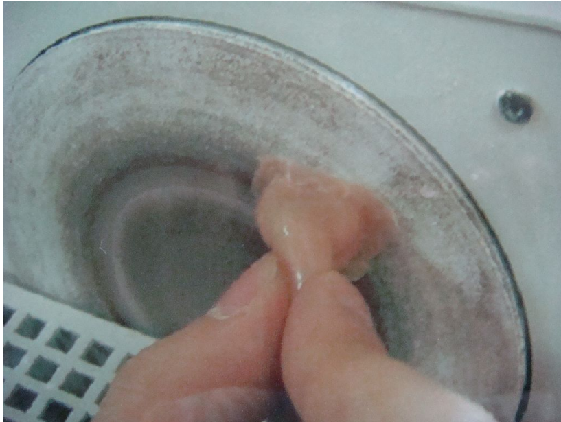
Figure 2 - 8 size down process. Grind the bottom edge of the ear shell using the grinder. The exact size of the ear shell is helpful to make the minimized hearing aid.
