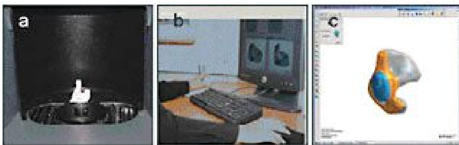
Figure 3 - 1 The 4 steps in manufacturing a CAD/CAM hearing aid shell (prior to final “printing” and assembling electronic components): a) An ear impression in a 3D scanner; b) The modeler makes changes to the virtual shell; c) View of the finished virtual hearing aid.
