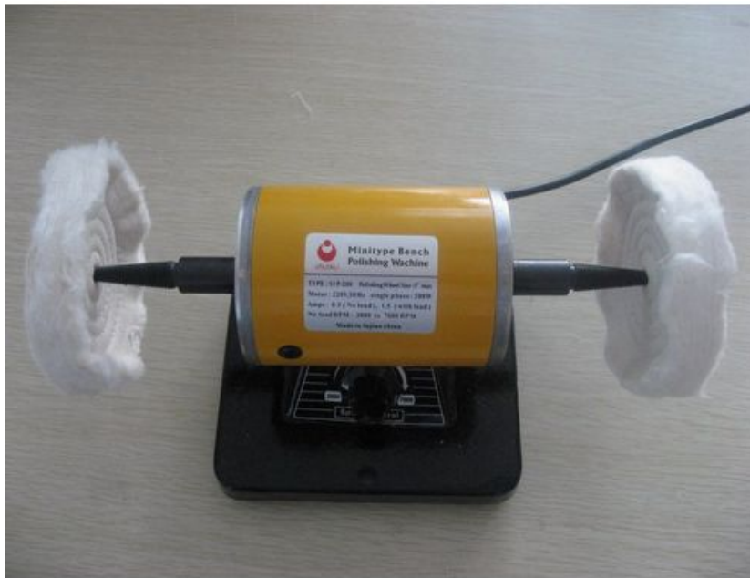
Figure 2 - 10 the polishing machine. The polishing machine is used for smoothing the ear shell and making the shell shinning.
