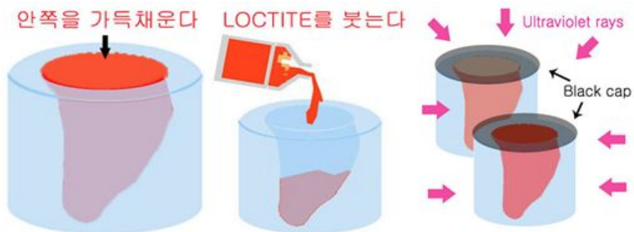
Figure 2 - 6 the curing process. First, pour the shell material into the investment; second, cover the investment with a black cap; then, put
