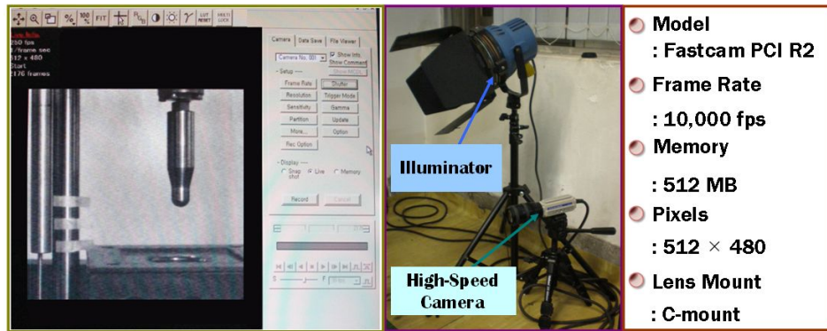
Fig. 5 Measurement of crash phenomenon between the drop head and specimen
