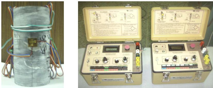
Figure 3.9 Strain gauge and portable strain indicator.
