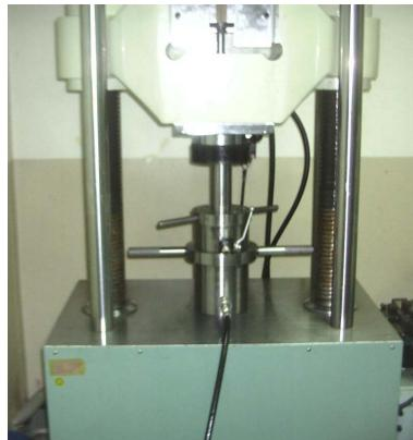
Figure 3.11 Triaxial compressive strength test.
