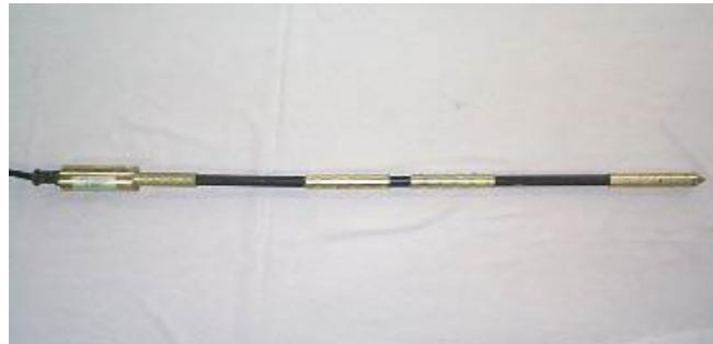
Figure 4.5 Rod extensometer (ER-4 m).
