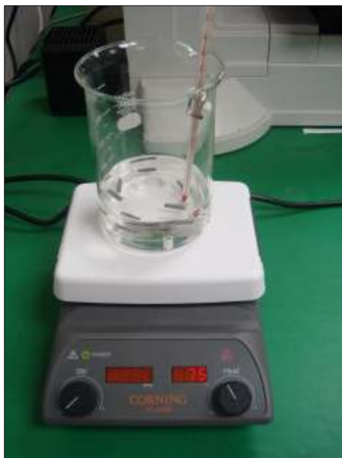
Photo. 3-4 Solvent extraction using N-hexan
