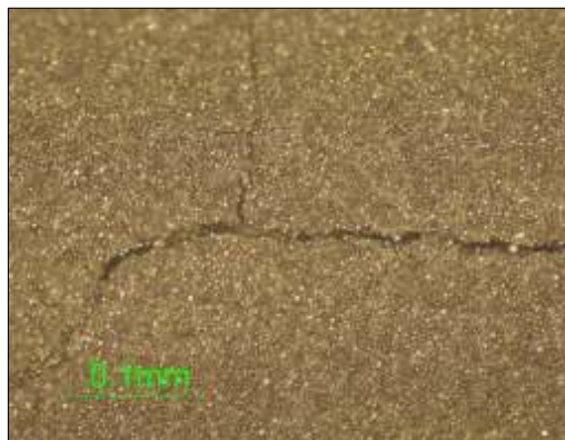
Photo. 4-1 Crack on green part during the solvent extraction at 55°C
