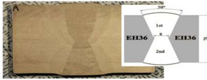
(b) Cross section of EGW welded specimen
