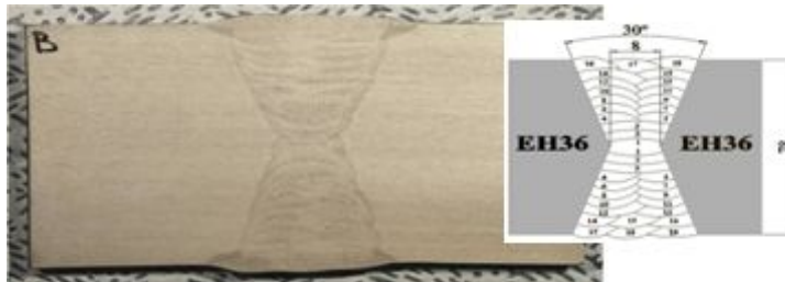
(c) Cross section of FCAW welded specimen
