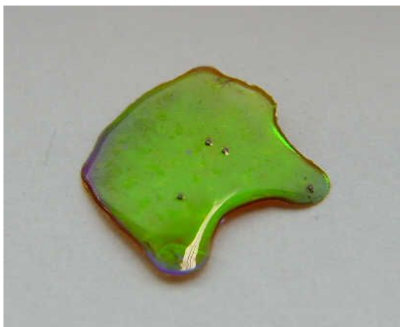
Figure 7.6. Photograph of polymer replica showing a reflection band at 534 nm.
