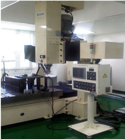
Fig. 3.1 WINXEN FSW equipment details
