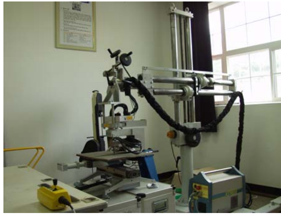
Fig. 4.5 Residual stress measurement machine(XRD)
