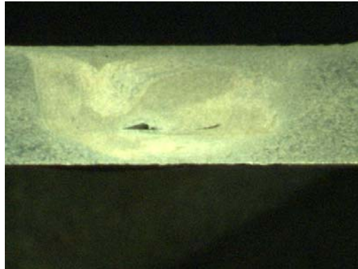
a) Cross section of similar welded specimen
