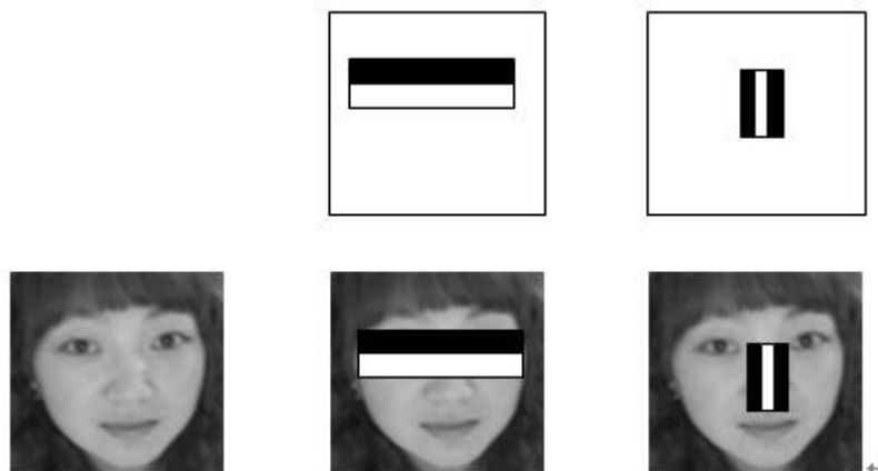
Fig. 4. Characteristic rectangles in 20 x 20 detector.
