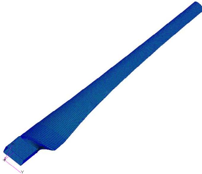
Fig. 18 Mesh generation for FEM analysis
