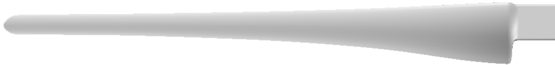
Fig. 9 Designed aerodynamic shape of 500W class wind turbine blade
