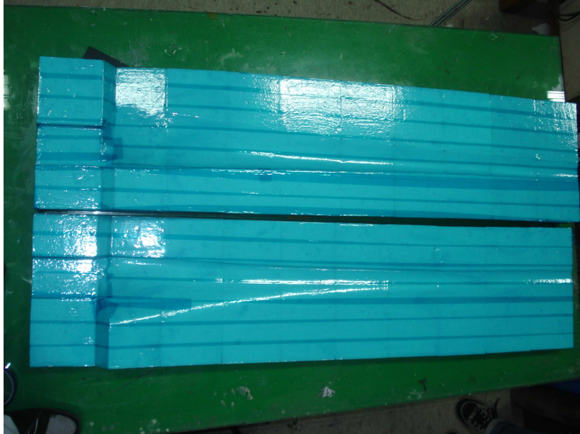
Fig. 37 Taping for gel coating
