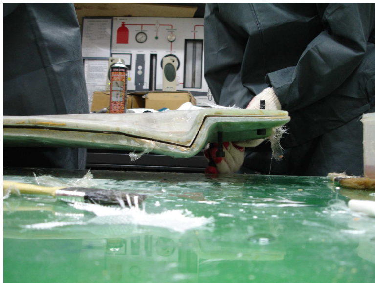
Fig. 40 Closed mold for curing
