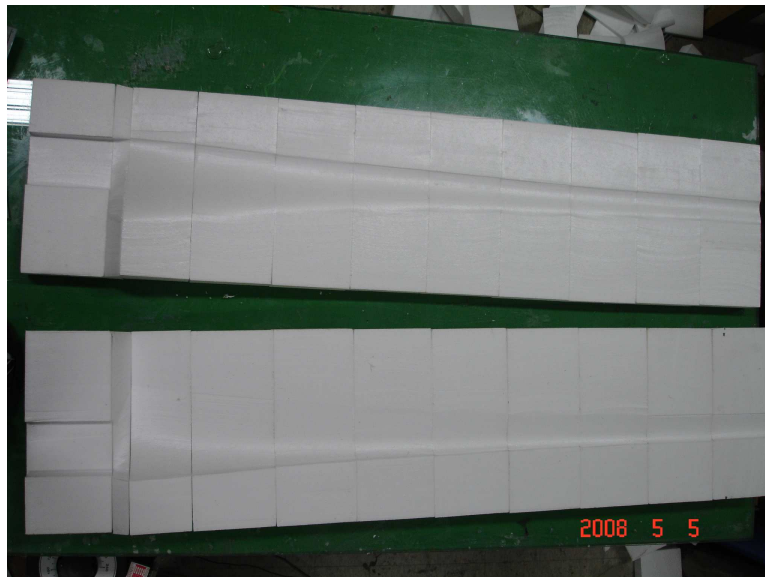
Fig. 36 Foam cutting for mold
