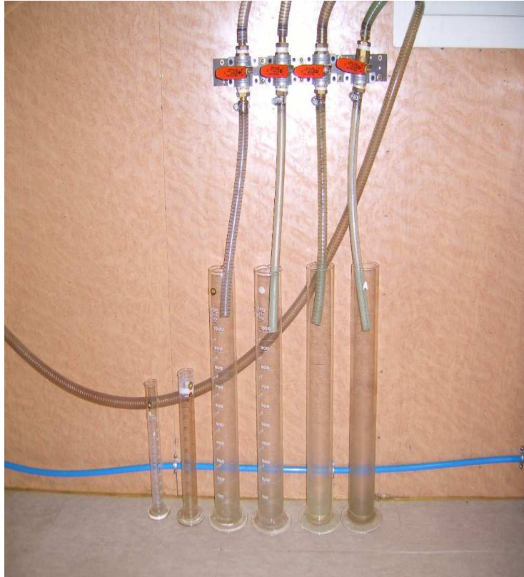
Photo. 3 Collection of Condensed Water
