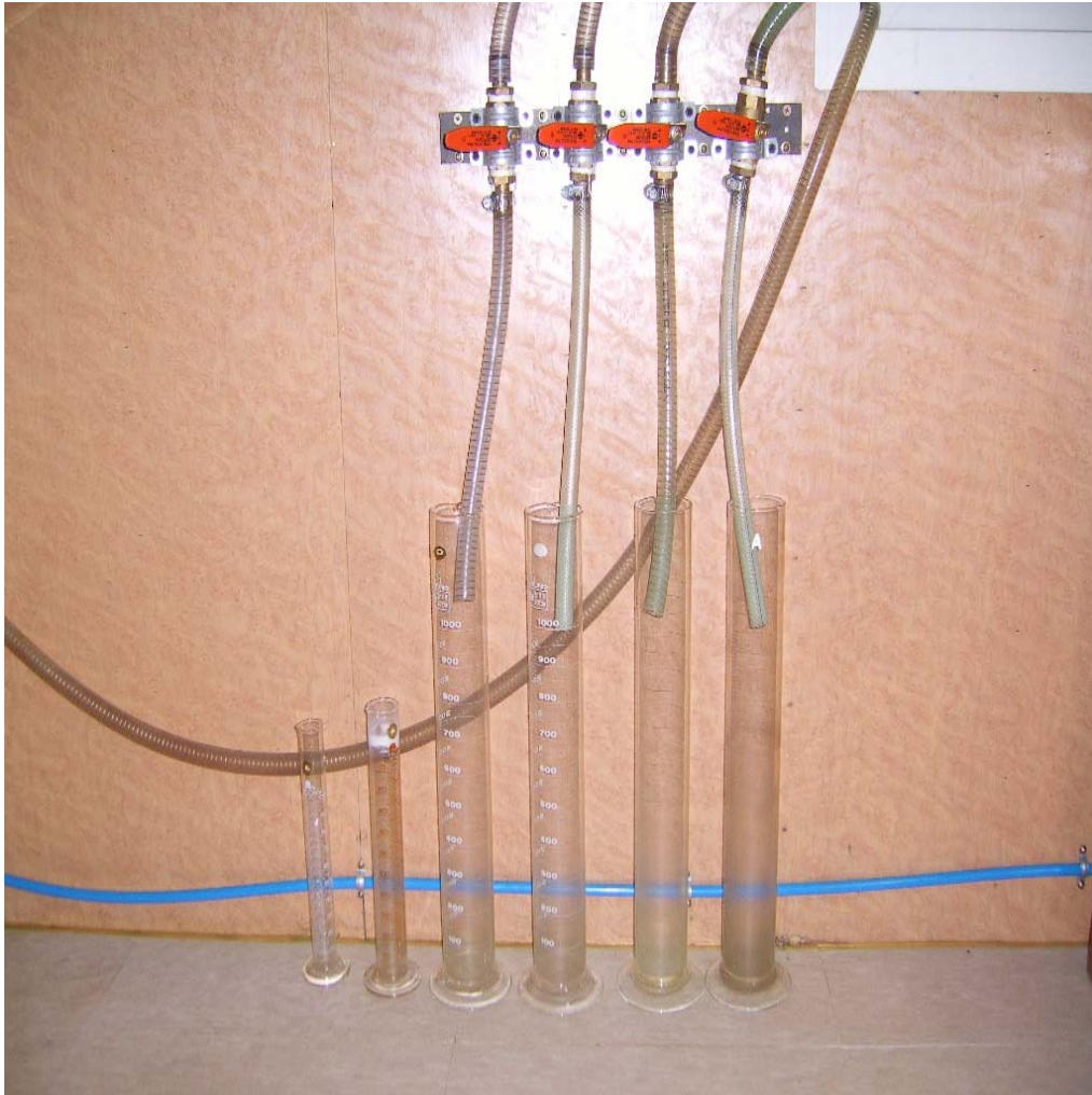
Photo.3 Collection of Condensed Water
