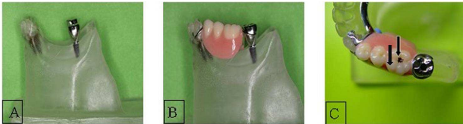
Fig. 8. Bilateral implant supported removable partial denture using clasp on the photoelastic epoxy resin model. A: prepared model, B: completed Akers type RPD, C: loading point(arrow).
