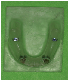
Fig. 7. Photoelastic epoxy resin model with resin teeth and dummy fixture.
