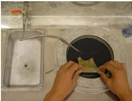
Fig. 17. Grinding of sliced specimen with rotating sand paper.
