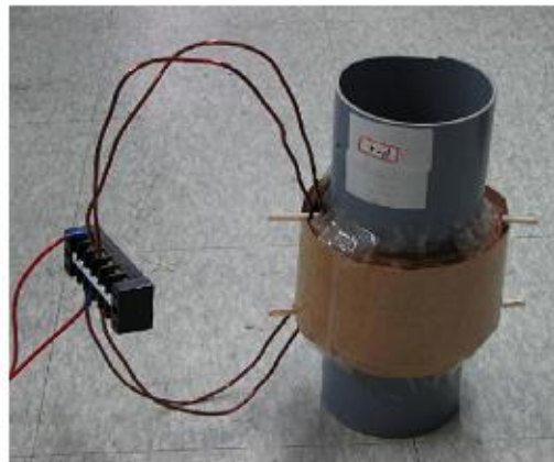
Fig. 17. The shunt coil in a current-limiting part
