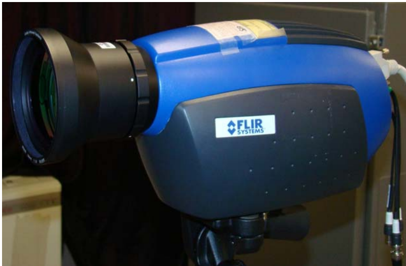
Fig. 3-5 Infrared Thermography Camera
