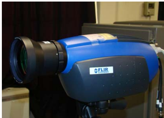
Fig 3-2 Infrared thermography system
