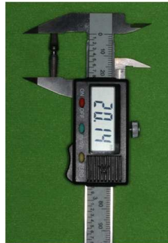
Fig.7. Caliper (Absolute Digimatic Caliper, Kawasaki, Japan) for measurement of implant length.
