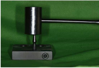
Fig.5. Tapping with a mallet.
