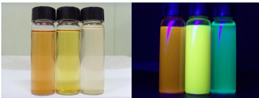
Fig. 3. Photoluminescence of CdSe nanocrystal
