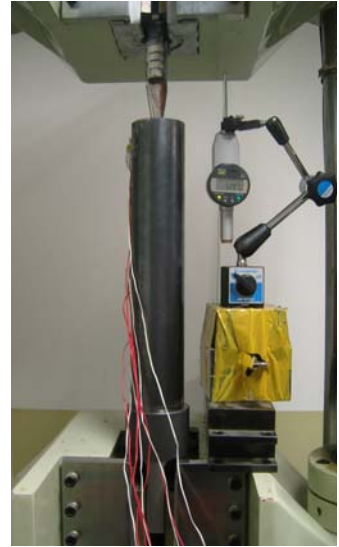
after pull-out test of spiral bolt
