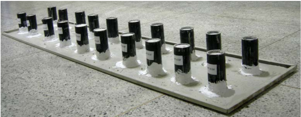
Figure 4-1. Curing of cylindrical specimens for uniaxial compression test.
