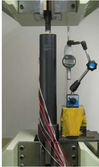
after pull-out test of rock bolt
