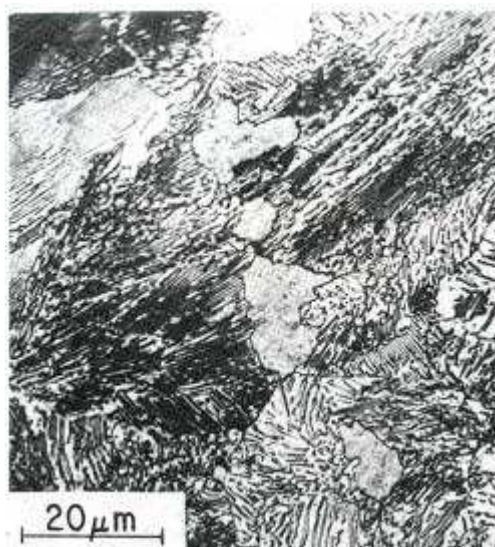
Fig. 2. 27. An optical micrograph showing the formation of austenite from pearlite along the boundary between pearlite colonies 33)~34) .
