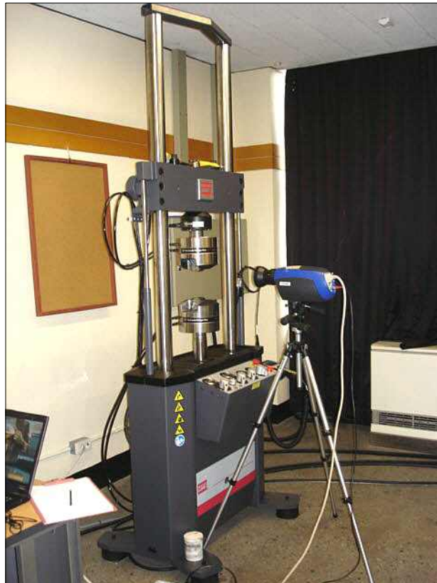
Fig. 4-4 Fatigue testing machine and InfraRed Thermography
