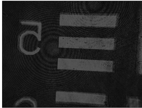
Fig. 5-5 Hologram image of resolution target(USAF1951)
