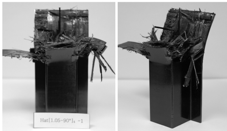
Photo. 20 Shape of collapsed CFRP side member. (Impact, \phi/\theta : 1.05/90^\circ )
