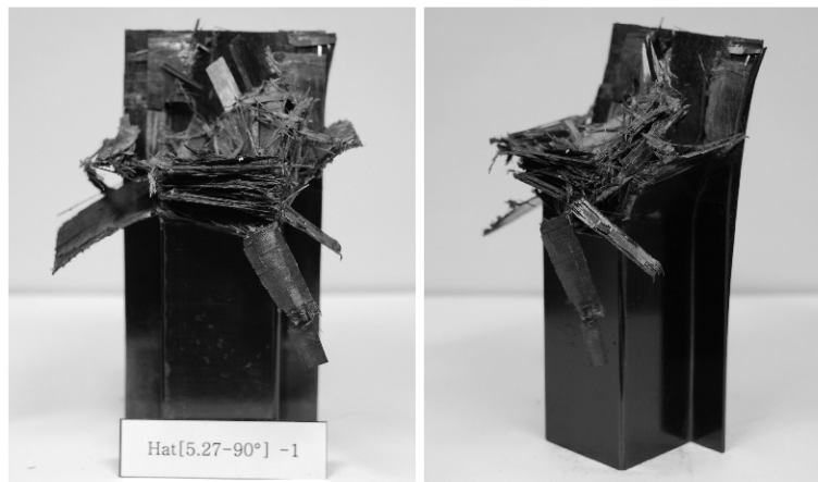
Photo. 22 Shape of collapsed CFRP side member. (Impact, \phi/\theta : 5.27/90^\circ )
