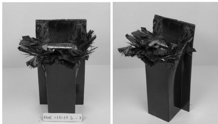
Photo. 23 Shape of collapsed Al/CFRP side member, [+15/-15] 4 (Impact, 15° fiber orientation angle)
