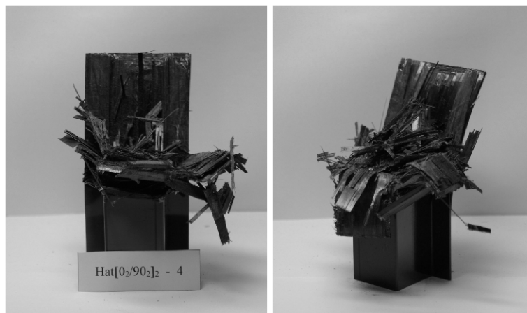
Photo. 13 Shape of collapsed CFRP side member, [0_2/90_2]_2 (Impact, 3 interface number)
