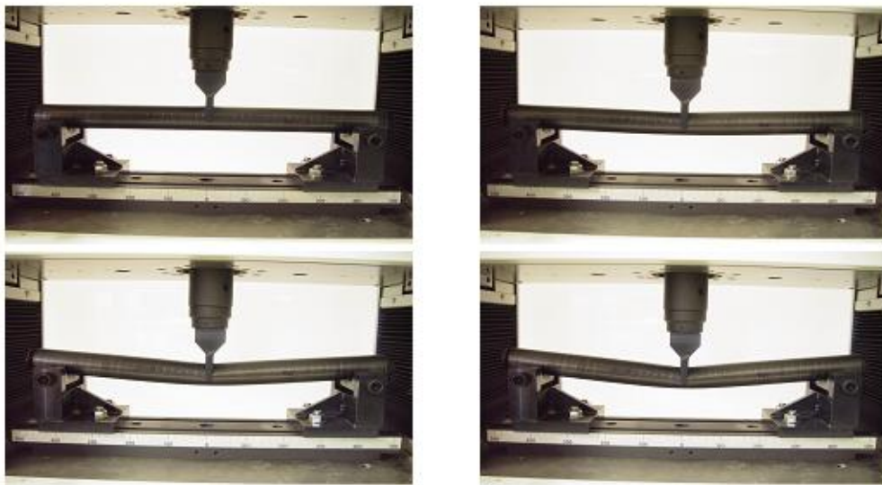
Photo. 30 Bending processing of HR [90° / 0°] 4
