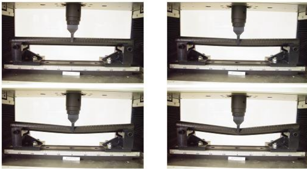
Photo. 26 Bending processing of HR[+15° / -15° ] 4
