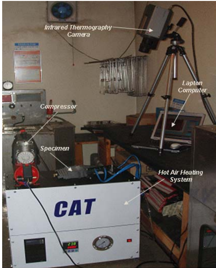
Fig. 2-16 Actual experiment equipment set
