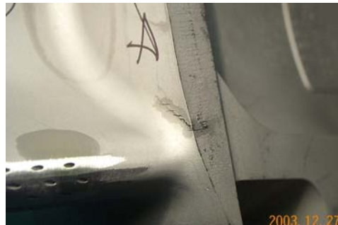
(d) Concave flatform crack (MS7001FA+e 1st stage bucket)
