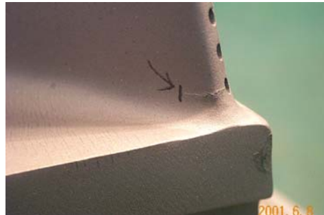
(f) Trailing edge cooling hold crack (MS7001FA 1st stage bucket)
