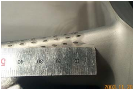
(e) Leading edge cooling hole crack (MS7001FA+e 1st stage bucket)
