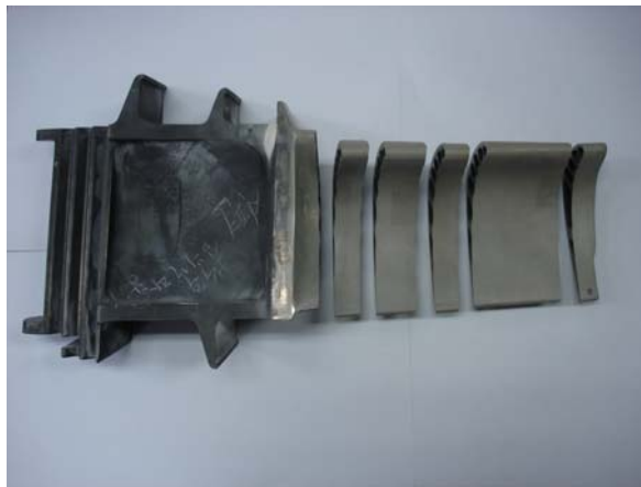
Fig. 2-26 Bucket as water jet cutting
