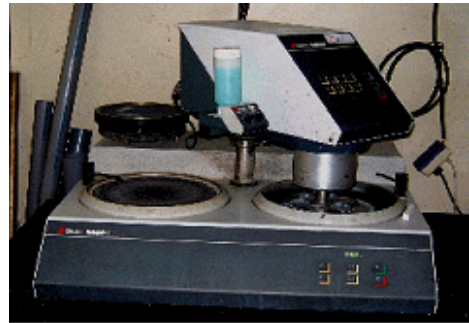
Fig. 3. Automatic specimen polisher (Rotapol 2, Struers, Denmark).
