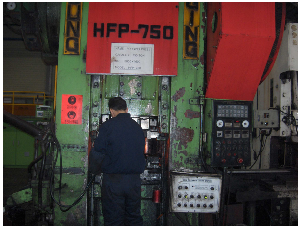
(a) Forging machine of 750ton
