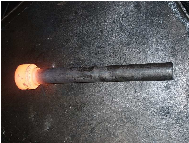
Fig. 3.18 First step forging part
