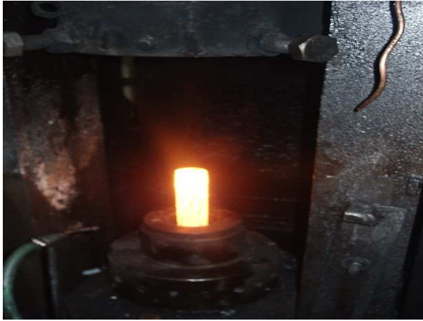
Fig. 3.15 Heating billet input
