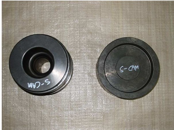
Fig. 3.21 First step forging molding
