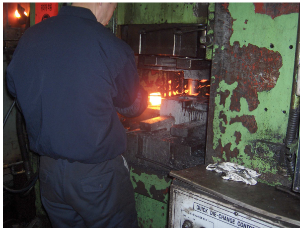
(b) Forging machine of 750ton
