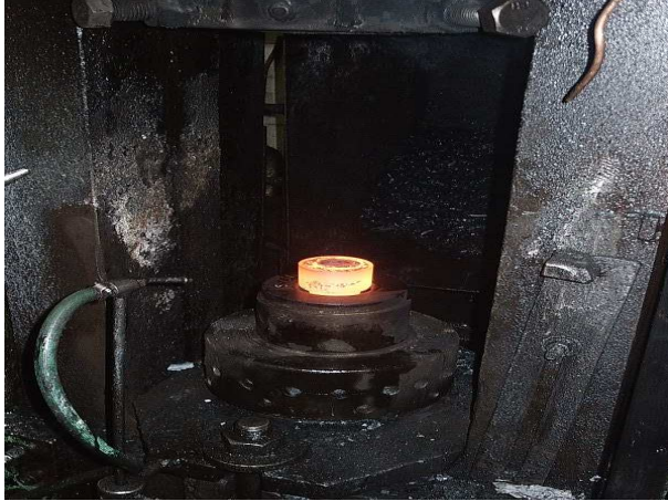
Fig. 3.17 First step forging
