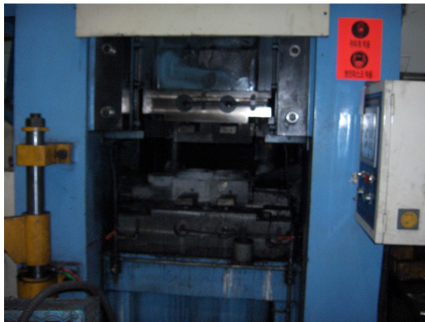
(b) Forging machine of 1300ton
