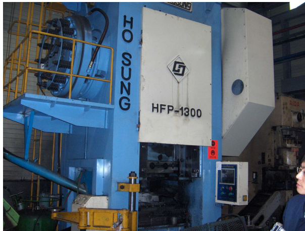
(a) Forging machine of 1300ton
