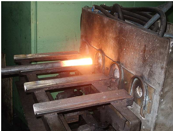
Fig. 3.14 Output of heating billet
