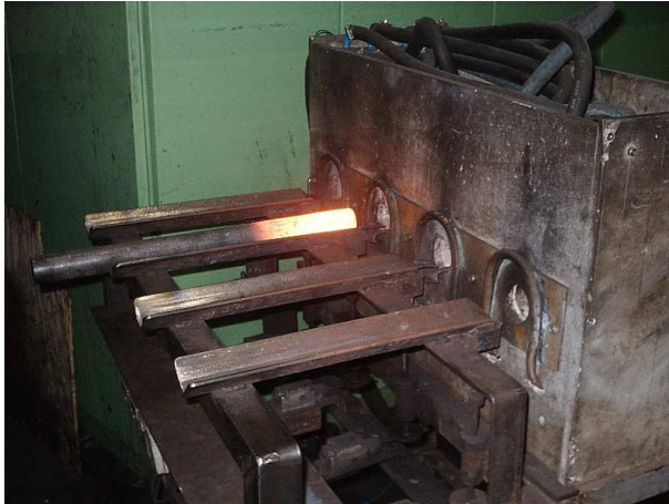
Fig. 3.13 Pull out of heating billet
