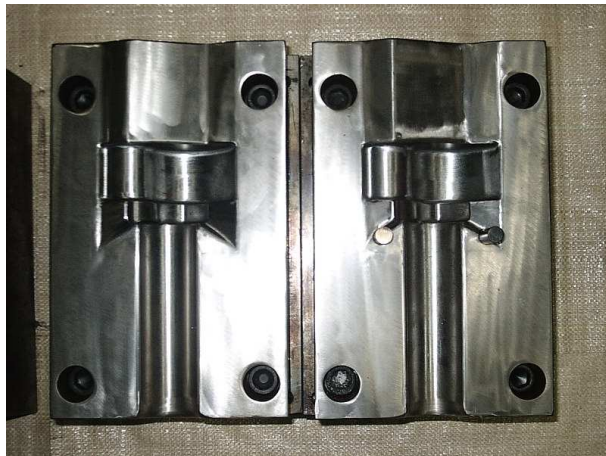
Fig. 3.22 Second step process forging molding
