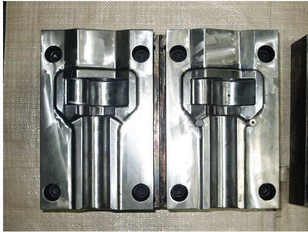
Fig. 3.23 Third step process forging molding
