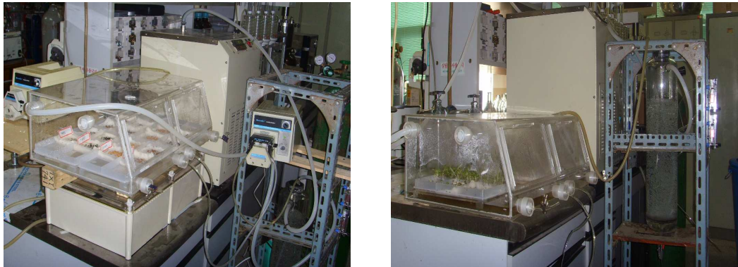
Fig. 4. Photographs of circulating oxygen water device.
