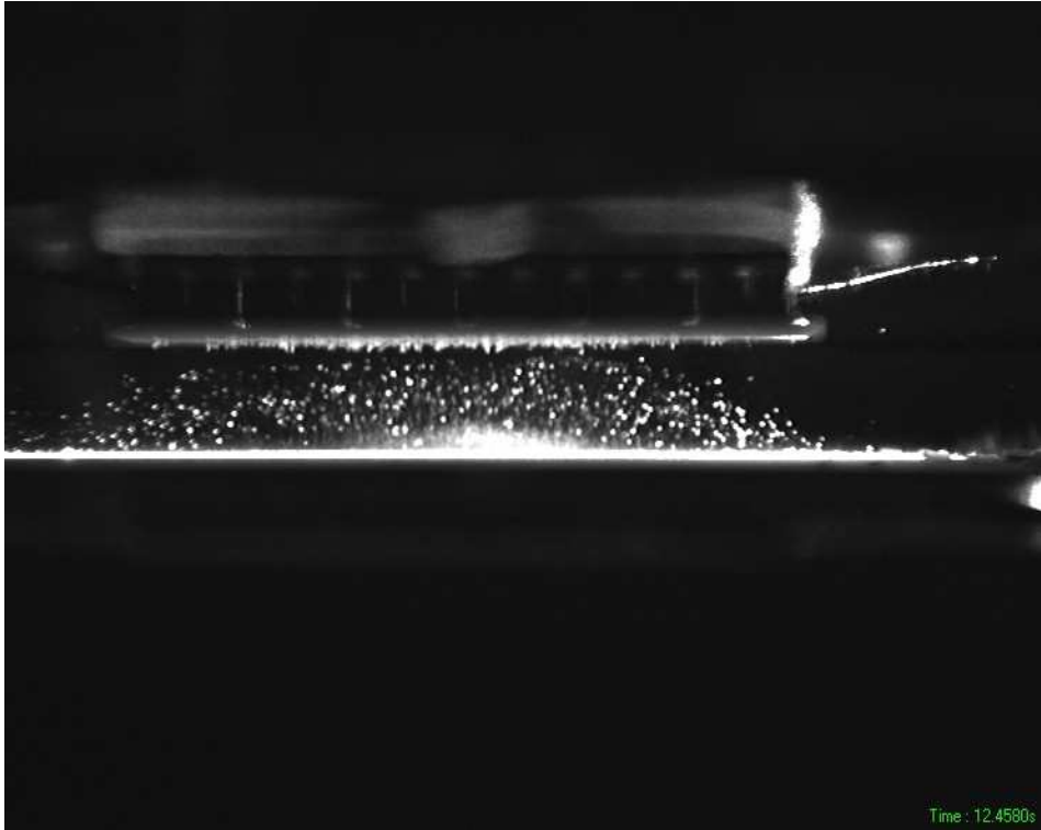
Fig. 22 Visualization of flow pattern at test section, only the piezoelectric actuators
