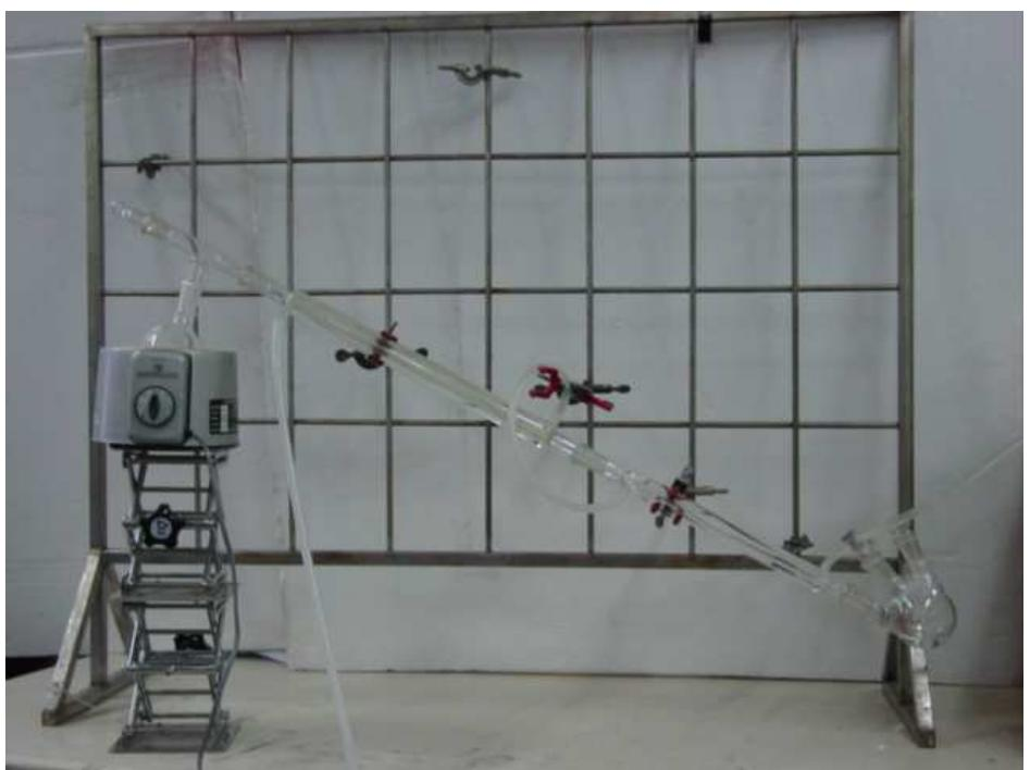
*Fig. 7. Distillatory apparatus for methanol extraction.*
