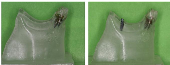
Fig. 7. Photoelastic epoxy resin model with resin teeth and dummy fixture.
