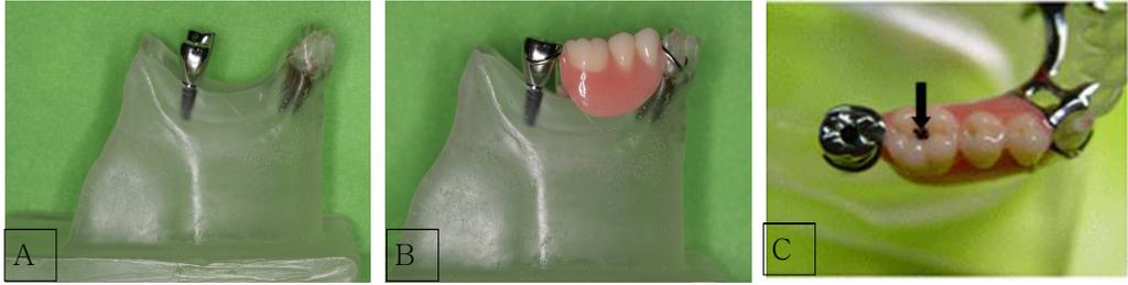
Fig. 9. Bilateral implant supported removable partial denture using clasp on the photoelastic epoxy resin model. A: prepared model, B: completed IRPD(Akers clasp), C: loading point(arrow).
