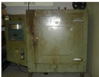
Fig. 12. Stress freezing furnace.
