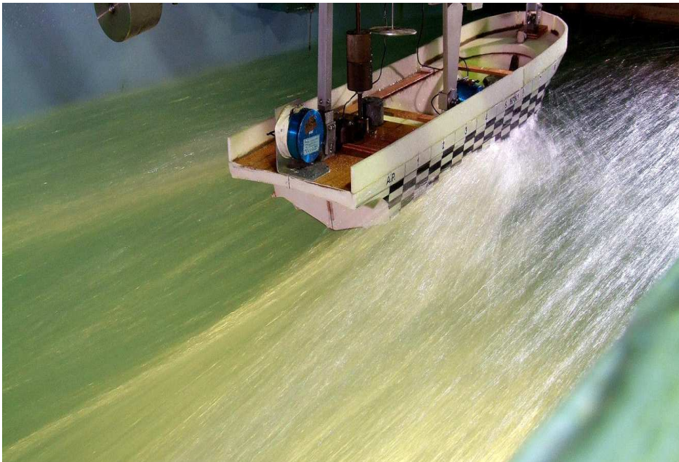
Photo 4.6 Wave Patterns for Case-3, V_s = 30.0 Knot
