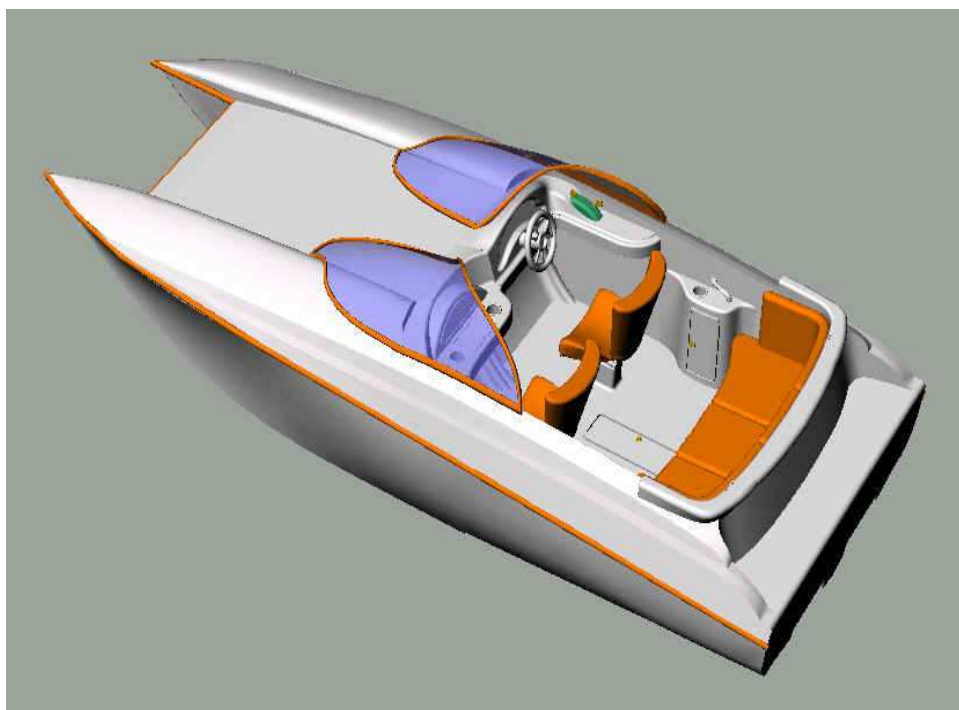
Fig. 6.13 3-D Design of Tunnel Type Powerboat
