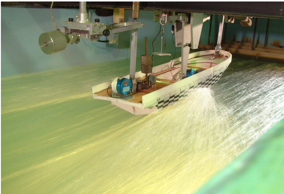
Photo 4.5 Wave Patterns for Case-2, V_s = 30.0 Knot
