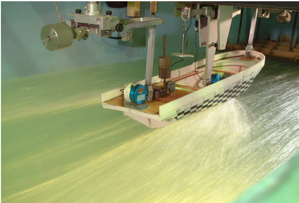
Photo 4.4 Wave Patterns for Case-1, V_s = 30.0 Knot
