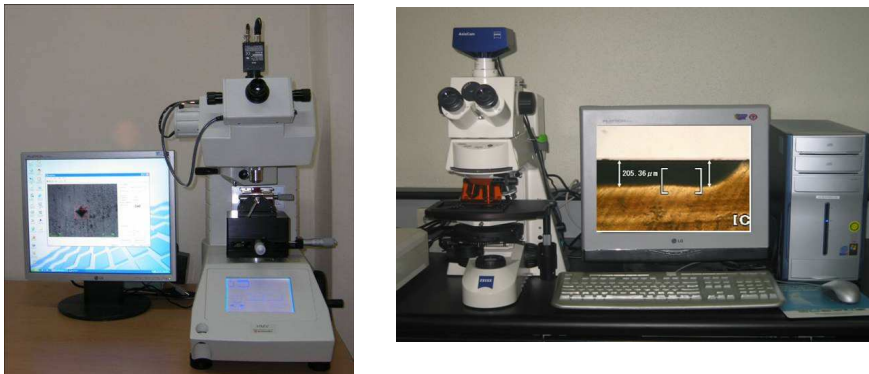
Fig.2. Surface microhardness tester (HMV-2 Shimadzu Co.,Japan) and Polarized light microscope (Axioskop 2 Plus, Zeiss, Germany)
