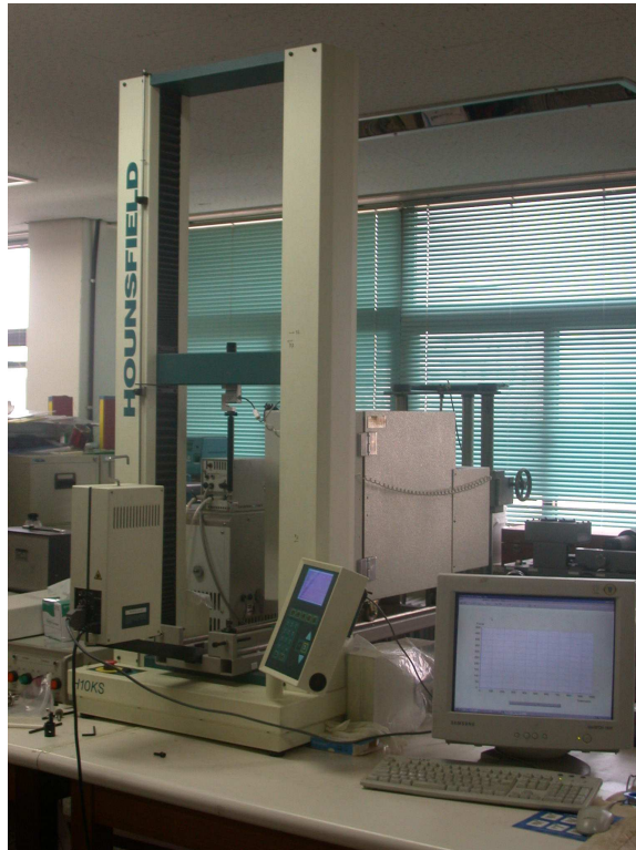
Fig. 3. 1. Photograph of universal test machine attached LASER extensometer.
