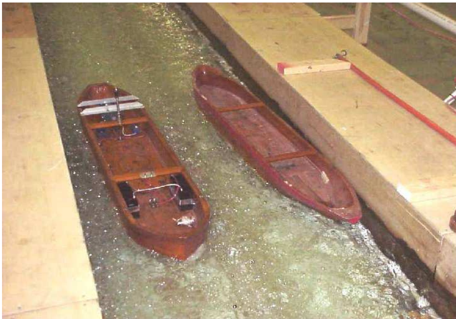
Fig. 23 Model M-RC(motor off) is following the eddy route in the channel and passing model M2 moored to the pier
