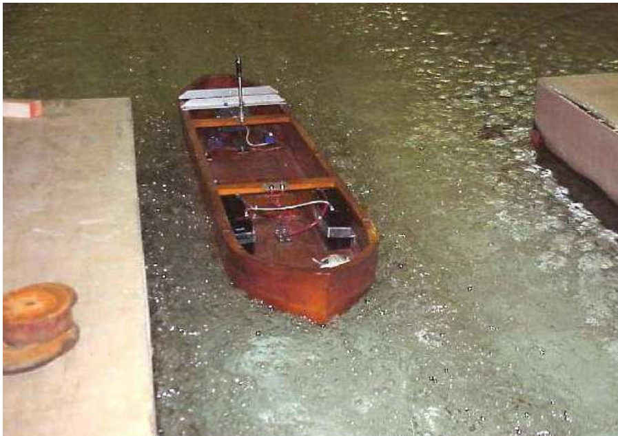
Fig. 22 Model M-RC (motor off) is coming in the channel following one of the eddy routes
