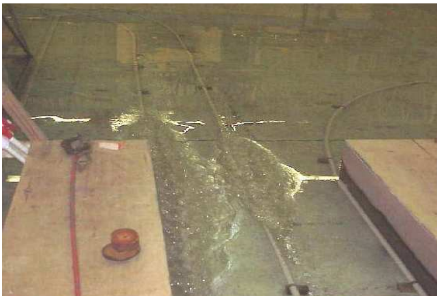
Fig. 20 The start of air injection into the water through the perforated pipes
