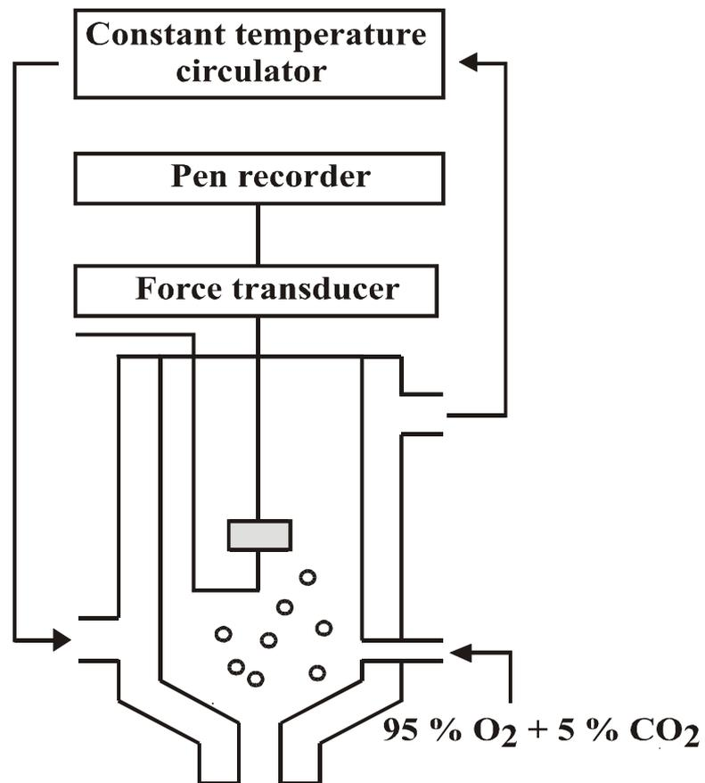
Fig. 1. A schematic representation of the recording system for isometric contraction with 15 mL tissue bath.
