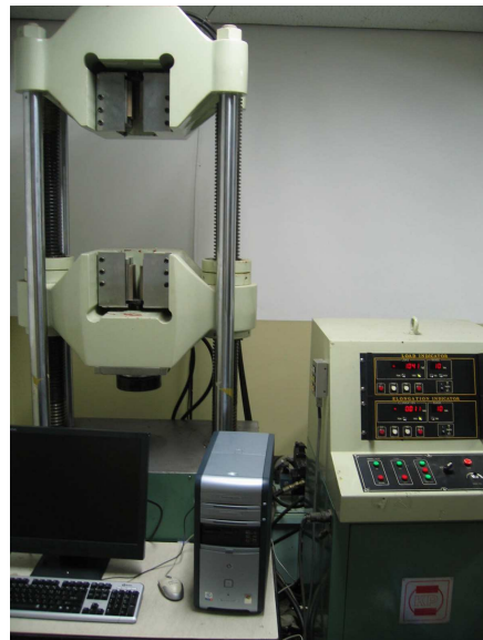
Figure 5-6. Schematic diagram for pull-out test of rock and spiral bolts and photography.
