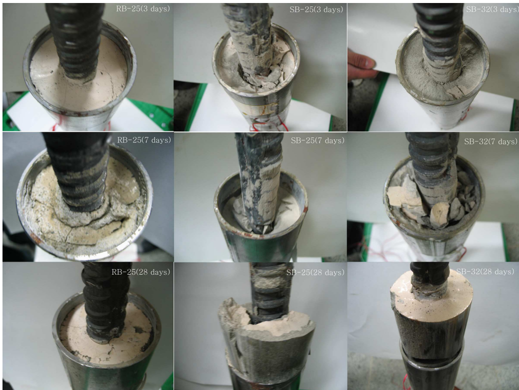
Figure 6-1. Pull-out test of rock and spiral bolts in laboratory.
