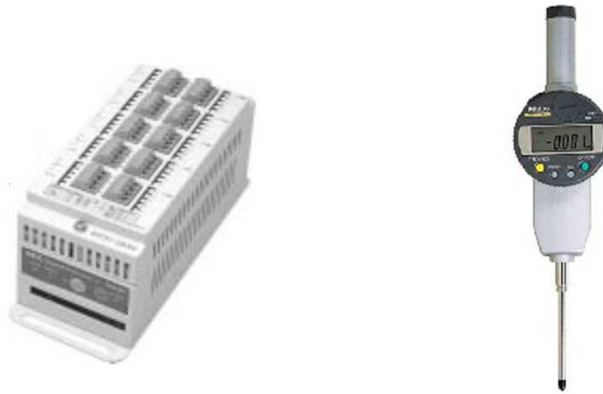
Figure 5-7. Data logger and digital displacement indicator used pull-out test of rock and spiral bolts.
