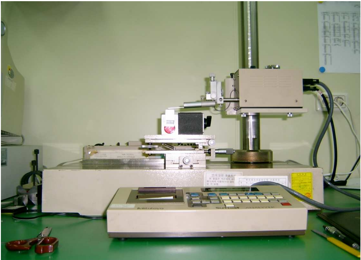
Fig. 15 Measuring equipment of surface roughness (Sufstest 402)
