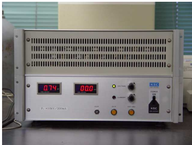
Fig. 3-11. Photograph of power supply for the NTP.
