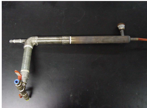
Fig. 3-15. Photograph of vapour generator.
