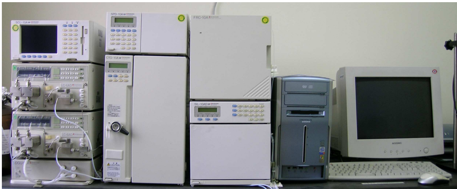
Figure 17. High performance liquid chromatography (HPLC) for determination of paclitaxel.
