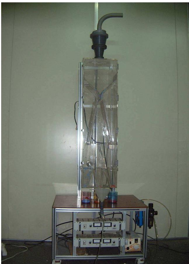
Fig. 18 Bench scale triboelectrostatic separator used in this study.
