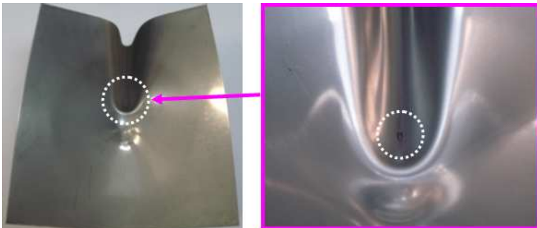
Fig. 38 Deformed shape of specimens for the case of drawing boundary conditions ( D=20 mm, E_{in}=45.7 J)
