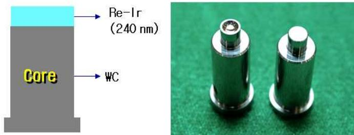
Fig. 3.30 Coating film structure and Re-Ir coated molding core
