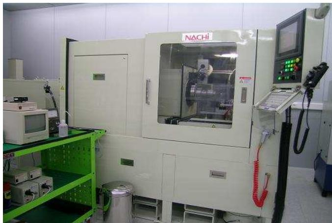
Photo 2.1 Microlens processing machine(ASP01, Nachi-Fujikoshi Co., Japan)
