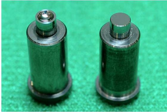
Photo 3.3 Molding core for aspheric glass lens
