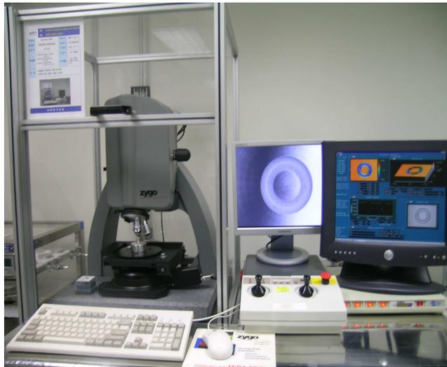
Photo 2.4 3-D surface roughness measurement system
