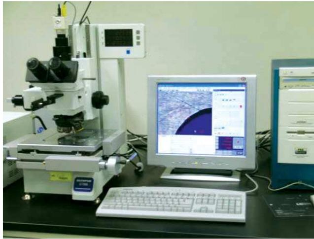
Photo 2.5 High precision vision inspection system(STM6, Olympus Co., Japan)
