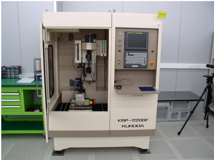
Photo 2.2 Aspheric polishing machine(KRP-2200F, Kuroda Co., Japan)
