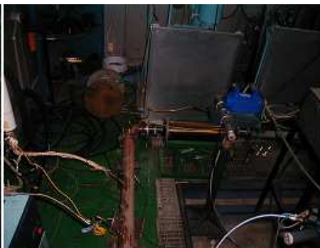
Fig. 3-12. Partial diesel particulate filter. Fig. 3-13. Installed PDPF.
