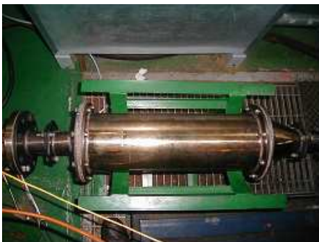
Fig. 3-12. Partial diesel particulate filter. Fig. 3-13. Installed PDPF.
