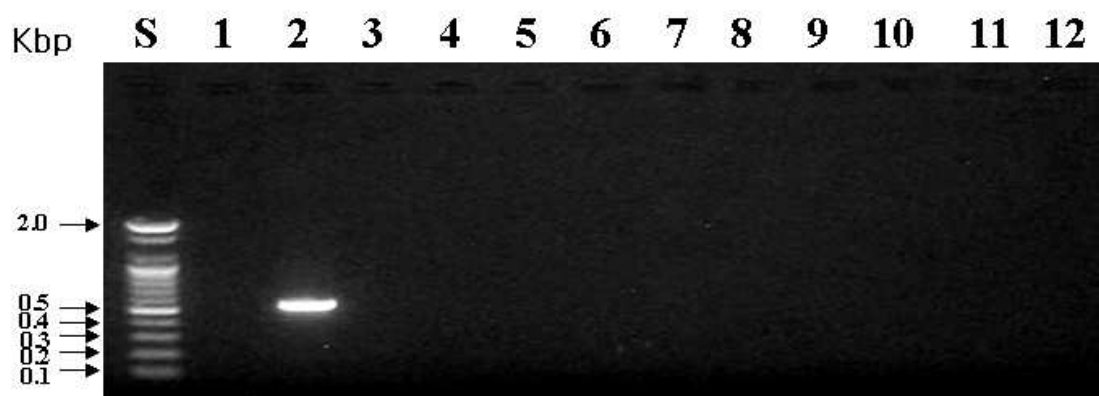
Fig. 2. Specificity test of PCR with ChDC–SsF2 and ChDC–SsR2 primers and purified genomic DNA of type strains.
