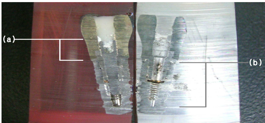
Fig. 18. OM showing the cross-sectioned surface morphology of the clinical used implant after potentiodynamic test. (a) abutment/fixture (b) fixture
